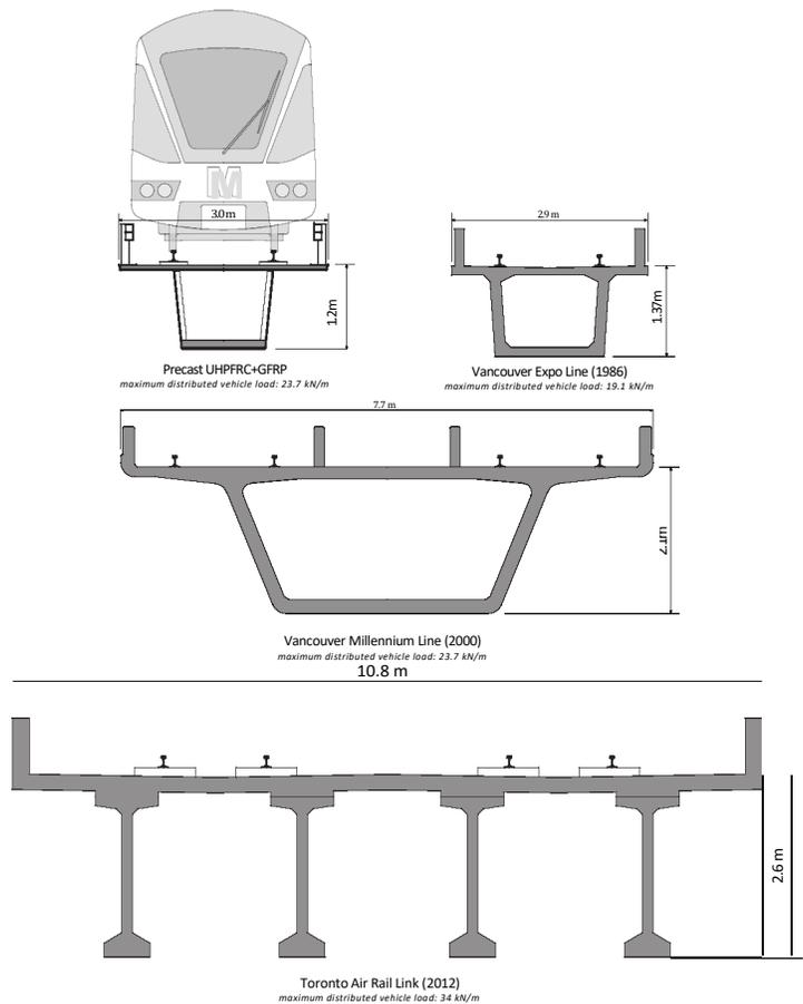
Comparison of guideway cross-sections for 33-37 m spans
