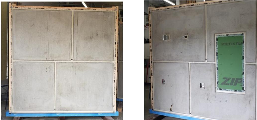
*Figure 1 : Photographs of both the opaque and penetrated single wythe precast test wall specimens*
